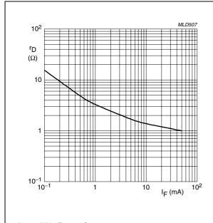
$f = 100 \text{ MHz}; T_j = 25 \,^{\circ}\text{C}.$
